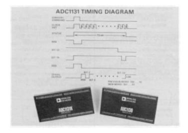
At this point the STATUS and CLOCK OUT return to Logic "0" and the conversion cycle ends.
