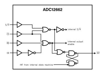
Figure 8. ADC Control Logic
