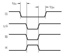
Figure 5.  $\overline{\text{CS}}$  Setup and Hold Timing for S/H,  $\overline{\text{RD}}$ , and OE
