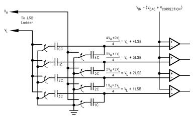
Figure 7. The Capacitive Voltage Divider
