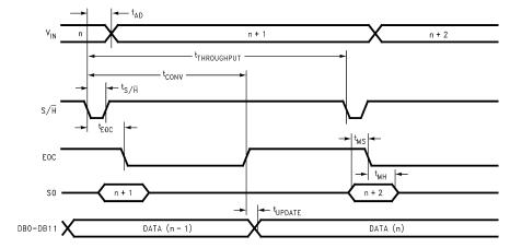
Figure 4. High Speed Interface Timing (MODE = 0, OE = 1,  $\overline{CS}$  = 0,  $\overline{RD}$  = 0)
