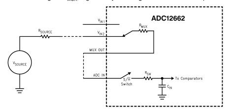
Figure 9. Simplified ADC12662 Input Stage
