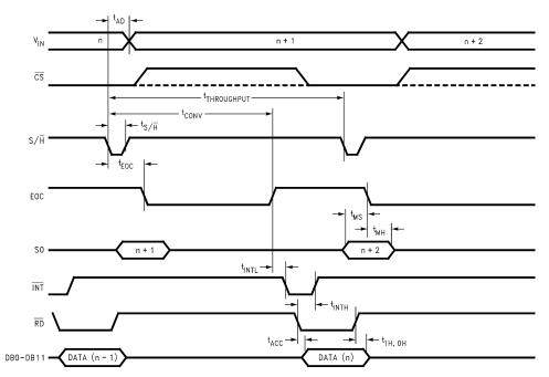
Figure 3. Interrupt Interface Timing (MODE = 0, OE = 1)
