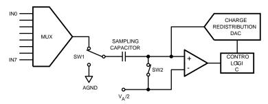
Figure 4. ADC128S102 in Track Mode
