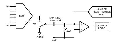
Figure 5. ADC128S102 in Hold Mode
