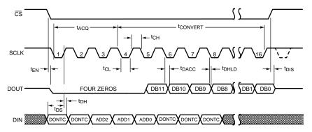
Figure 2. ADC128S102 Serial Timing Diagram
