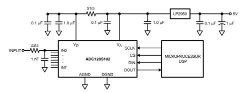
Figure 8. Typical Application Circuit
