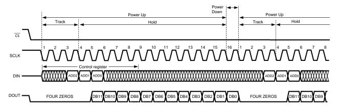
Figure 1. ADC128S102 Operational Timing Diagram
