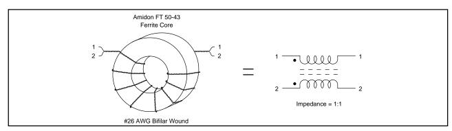
FIGURE 7. Common-Mode Choke Transformer Windings.
