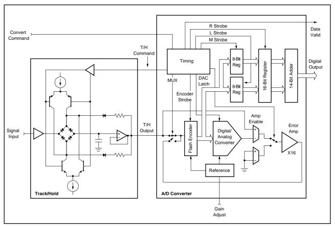
FIGURE 1. ADC614 Block Diagram—A Two-Step Subranging Architecture.
