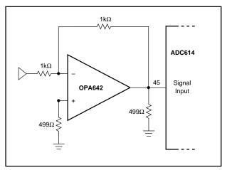
FIGURE 8. Single Ended Input Amplifier (Gain = -1V/V).
