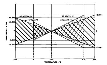
Figure 2. AD ADC72 Gain Drift Error vs. Temperature
