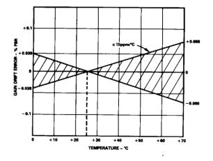
Figure 3. AD ADC71 Gain Drift Error vs. Temperature
