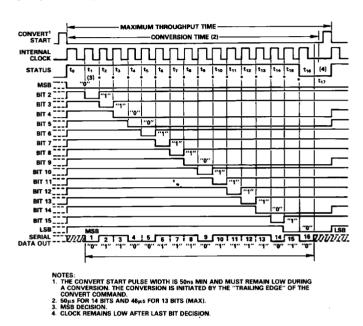
Figure 8. Timing Diagram (Binary Code 0110011101111010)
