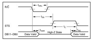
FIGURE 1. R/C Pulse Low—Outputs Enabled After Conversion.
