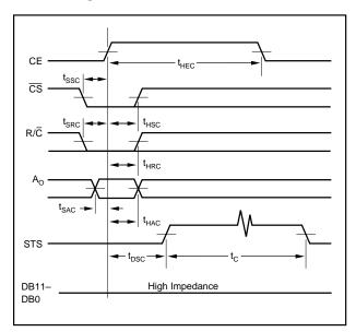
FIGURE 3. Conversion Cycle Timing.
