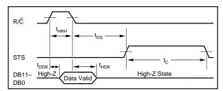
FIGURE 2.  $R/\overline{C}$  Pulse High—Outputs Enabled Only While  $R/\overline{C}$  Is High.
