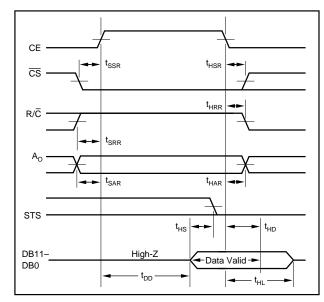
FIGURE 4. Read Cycle Timing.
