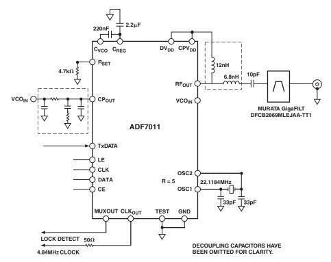
Figure 17. Application Diagram — 868 MHz Operation with +10 dBm Output Power
