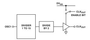
Figure 3. CLK<sub>OUT</sub> Stage
