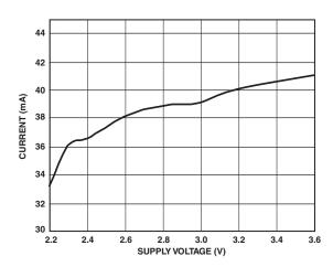
TPC 12.  $I_{DD}$  vs.  $V_{DD}$  @ 10 dBm
