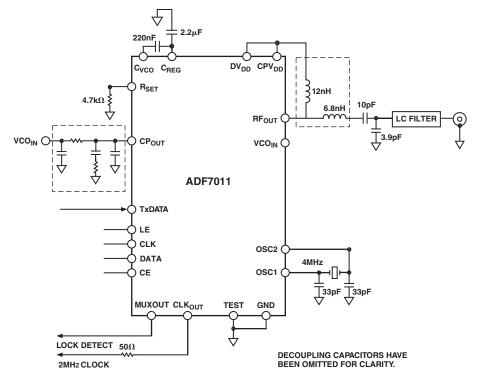
Figure 15. Application Diagram – 433 MHz Operation with +10 dBm Output Power
