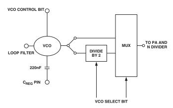
Figure 7. Voltage Controlled Oscillator
