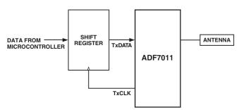
Figure 14. TxCLK Pin Synchronizing Data for GFSK
