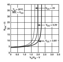
TPC 1. On Resistance vs. Input Voltage
