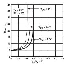
TPC 3. On Resistance vs. Input Voltage
