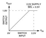
Figure 8. 2.5 V to 1.8 V Voltage Translation,  $\overline{SEL} = V_{CC}$
