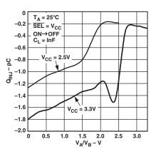
TPC 12. Charge Injection vs. Source Voltage
