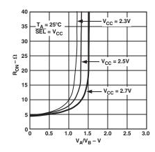
TPC 2. On Resistance vs. Input Voltage
