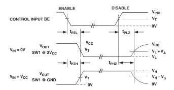
Figure 3. Enable and Disable Times
