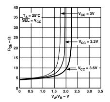
TPC 1. On Resistance vs. Input Voltage
