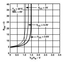
TPC 3. On Resistance vs. Input Voltage
