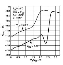
*TPC 12. Charge Injection vs. Source Voltage*
