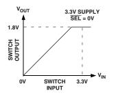
Figure 10. 3.3 V to 1.8 V Voltage Translation, SEL = 0 V
