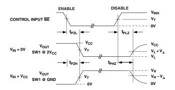
Figure 3. Enable and Disable Times
