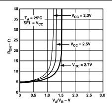
TPC 2. On Resistance vs. Input Voltage
