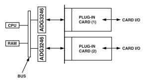
Figure 12. ADG3246 in a Hot Plug Application
