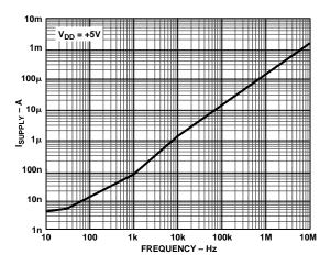
Figure 4. Supply Current vs. Input Switching Frequency
