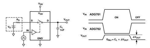
Test Circuit 5. Charge Injection
