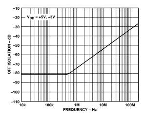
Figure 5. Off Isolation vs. Frequency
