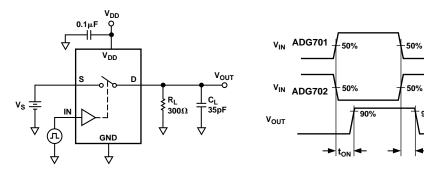
Test Circuit 4. Switching Times
