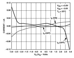
Figure 8. Leakage Currents as a Function of V<sub>D</sub> (V<sub>S</sub>)
