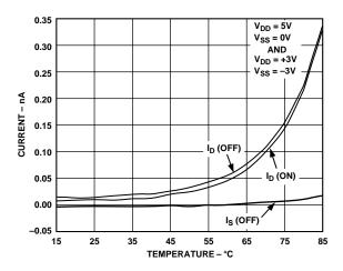
Figure 9. Leakage Currents as a Function of Temperature
