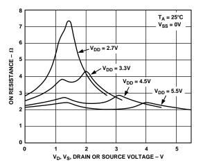
Figure 1. On Resistance as a Function of  $V_{\text{D}}$  (V\_{\text{S}}) for Single Supply
