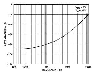
Figure 12. Off Isolation vs. Frequency
