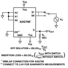
Test Circuit 9. OFF Isolation and Bandwidth
