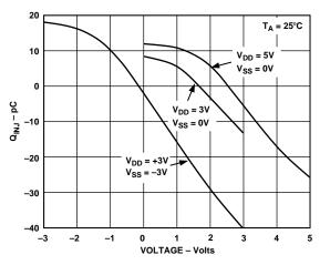
Figure 15. Charge Injection vs. Source Voltage
