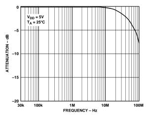
Figure 14. On Response vs. Frequency
