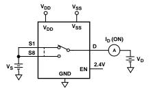
Test Circuit 4. I<sub>D</sub> (ON)
