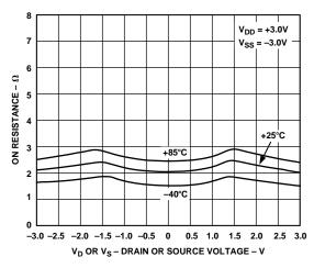
Figure 5. On Resistance as a Function of  $V_D$  ( $V_S$ ) for Different Temperatures, Dual Supply
