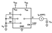
Test Circuit 3. I<sub>D</sub> (OFF)
