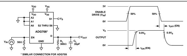
Test Circuit 7. Enable Delay, t<sub>ON</sub> (EN), t<sub>OFF</sub> (EN)
