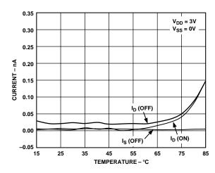
Figure 10. Leakage Currents as a Function of Temperature
