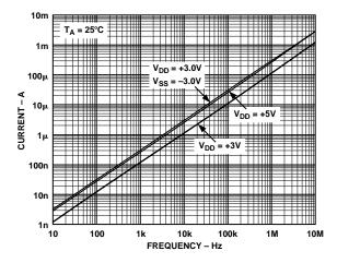
Figure 11. Supply Current vs. Input Switching Frequency
