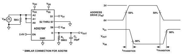
Test Circuit 5. Switching Time of Multiplexer, t<sub>TRANSITION</sub>
