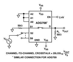
Test Circuit 10. Channel-to-Channel Crosstalk
