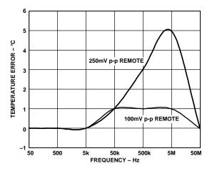
Figure 3. Temperature Error vs. Power Supply Noise Frequency
