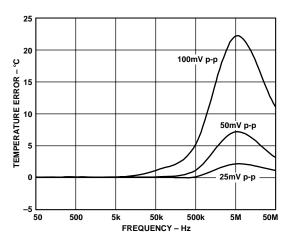
Figure 4. Temperature Error vs. Common-Mode Noise Frequency
