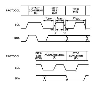
Figure 1. Diagram for Serial Bus Timing
