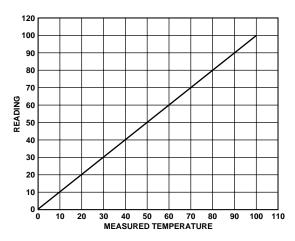
*Figure 5. Pentium II Temperature Measurement vs. ADM1021 Reading*
