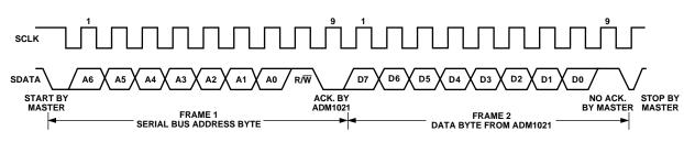
Figure 15. Reading Data from a Previously Selected Register
