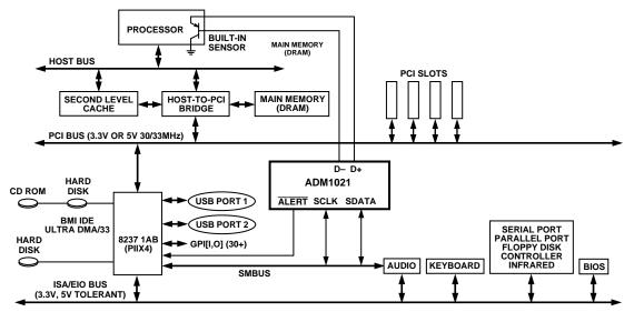
Figure 19. Typical System Using ADM1021
