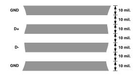
Figure 17. Arrangement of Signal Tracks
