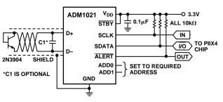
Figure 18. Typical ADM1021 Application Circuit
