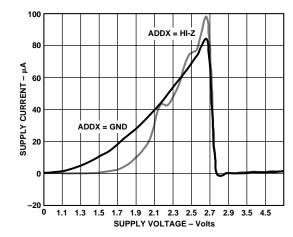
Figure 10. Standby Supply Current vs. Supply Voltage
