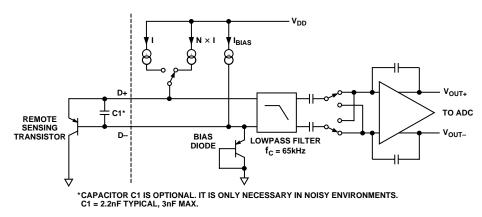
Figure 12. Input Signal Conditioning
