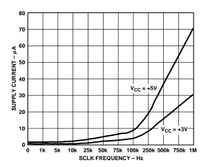
Figure 7. Standby Supply Current vs. Clock Frequency
