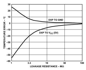
Figure 2. Temperature Error vs. PC Board Track Resistance
