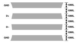
Figure 12. Arrangement of Signal Tracks
