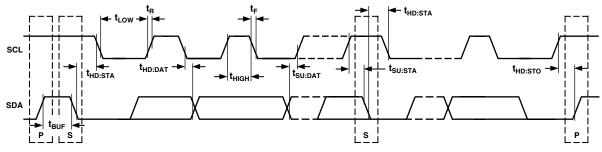
Figure 1. Diagram for Serial Bus Timing
