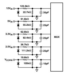
Figure 10. Structure of Analog Inputs
