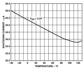
Figure 8. Standby Current vs. Temperature
