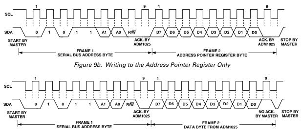
Figure 9c. Reading Data from a Previously Selected Register
