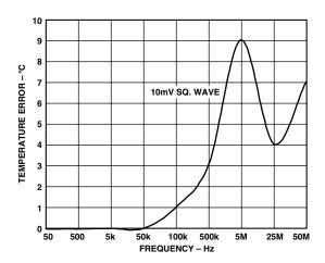
*Figure 7. Temperature Error vs. Differential-Mode Noise Frequency*
