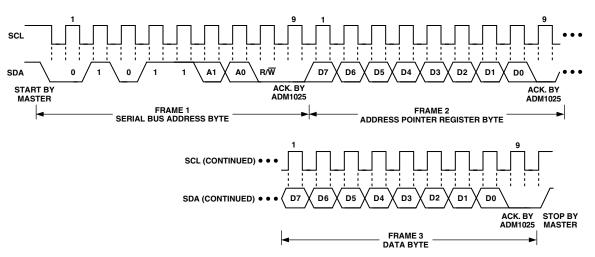
Figure 9a. Writing a Register Address to the Address Pointer Register, then Writing Data to the Selected Register
