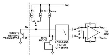
Figure 11. Signal Conditioning for External Diode Temperature Sensors
