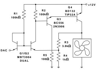
Figure 10f. Discrete Fan Drive Circuit with Bipolar Output Dual Supply
