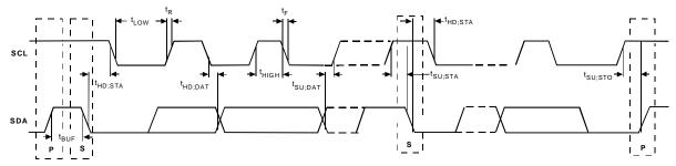
Figure 1. Diagram for Serial Bus Timing
