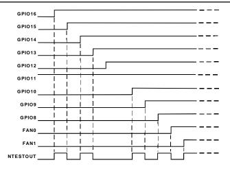
Figure 25. NAND Tree Test With One Input Stuck High
