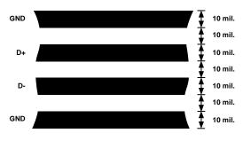
Figure 9. Arrangement of Signal Tracks
