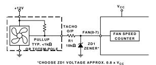
Figure 12c. Fan with Strong Tach. Pullup to >V<sub>cc</sub> or Totem-Pole Output, Clamped with Zener and Resistor
