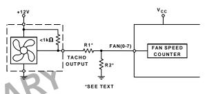
Figure 12d. Fan with Strong Tach. Pullup to >V<sub>cc</sub> or Totem-Pole Output, Attenuated with R1/R2
