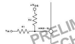
Figure 6. Scaling and Offsetting AIN(0 - 9) for Negative Inputs
