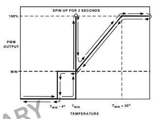
Figure 11a. Automatic PWM Fan Control Transfer Function
