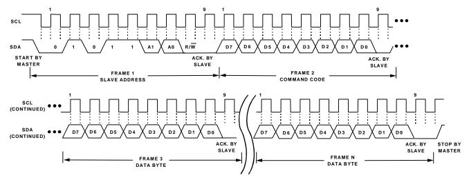
Figure 2a. General SMBus Write Timing Diagram
