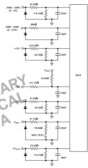
Figure 4. Structure of Analog Inputs
