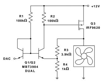
Figure 10d. Discrete Fan Drive Circuit with P-Channel MOSFET, SIngle Supply
