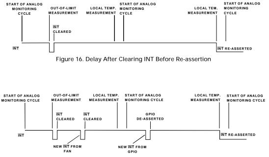
Figure 17. Other Interrupt Sources Can Re-assert INT Immediately
