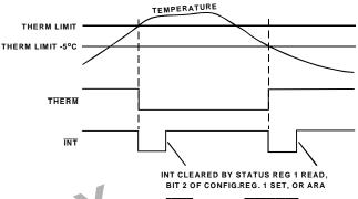
Figure 19. Assertion Of INT Due To THERM Event
