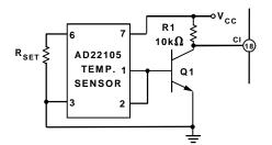
Figure 14. Using the CI Input with a Temperature Sensor
