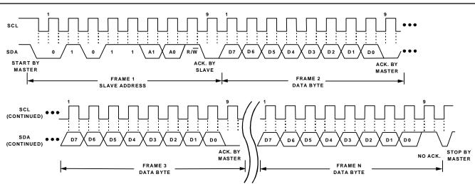
Figure 2b. General SMBus Read Timing Diagram
