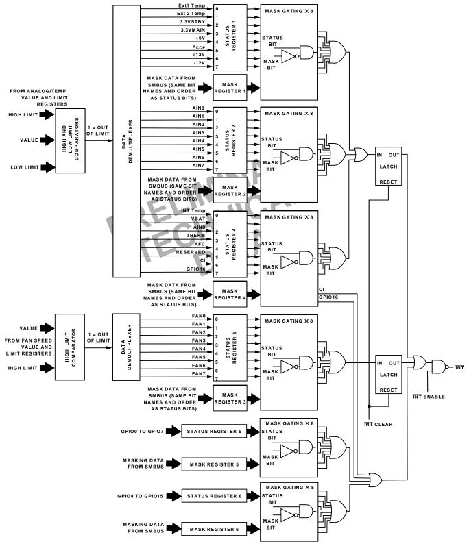
Figure 15. ADM1026 Interrupt Structure
