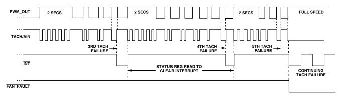
Figure 22. Operation of FAN\_FAULT and Interrupt Pins
