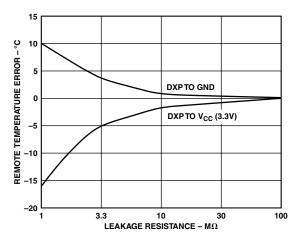
TPC 1. Temperature Error vs. PCB Track Resistance
