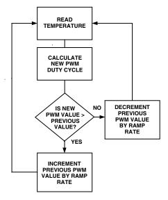
Figure 12. Filtered Mode Algorithm
