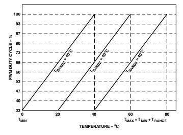
Figure 8. Effect of Increasing T<sub>MIN</sub> Value on Control Loop
