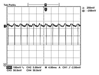
Figure 20. Fan Speed Sensing Waveform at TACH/AIN Pin
