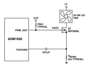
Figure 19. Interfacing the ADM1030 to a 2-Wire Fan
