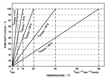
Figure 7. PWM Duty Cycle vs. Temperature Slopes (T<sub>RANGE</sub>)
