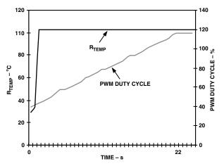
Figure 14. Filtered Mode with Ramp Rate = 4
