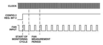
Figure 21. Fan Speed Measurement
