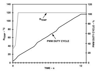
Figure 13. Filtered Mode with Ramp Rate = 8
