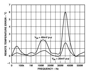
TPC 3. Temperature Error vs. Common-Mode Noise Frequency
