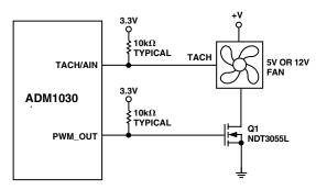
Figure 18. Interfacing the ADM1030 to a 3-Wire Fan
