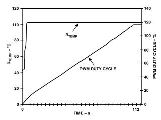
Figure 16. Filtered Mode with Ramp Rate = 1
