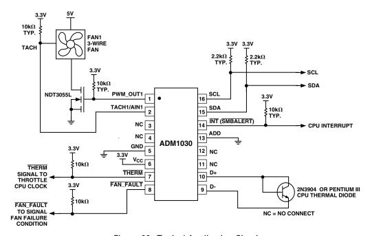
Figure 23. Typical Application Circuit
