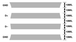
Figure 4. Arrangement of Signal Tracks
