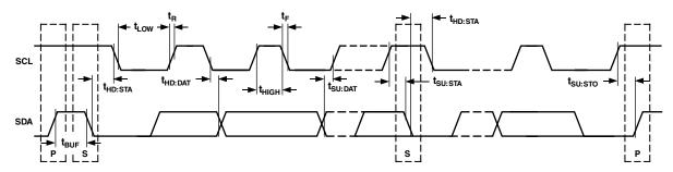
Figure 1. Diagram for Serial Bus Timing
