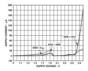
TPC 8. Standby Supply Current vs. Supply Voltage
