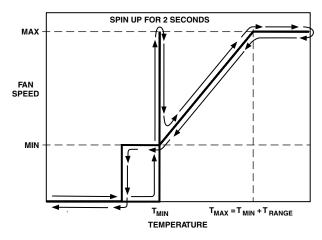
Figure 6. Automatic Fan Speed Control
