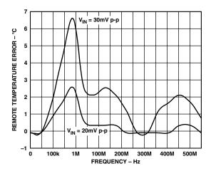
TPC 7. Temperature Error vs. Differential-Mode Noise Frequency
