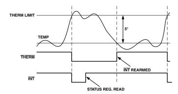
Figure 5. Operation of THERM and INT Signals
