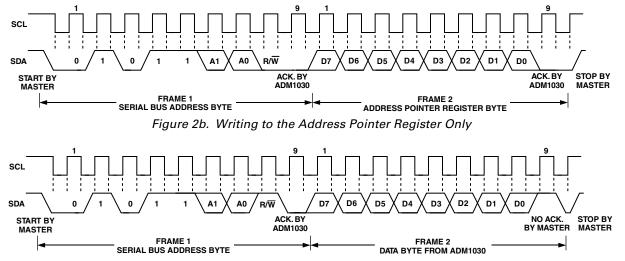
Figure 2c. Reading Data from a Previously Selected Register
