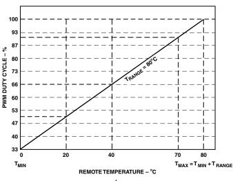
Figure 9. Max Speed Calculated by Local and Remote Temperature Control Loops Drives Fan
