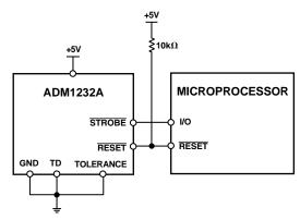
Figure 1. Typical Supply Monitoring Application
