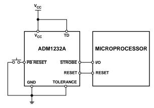
Figure 2. Typical Push Button Reset Application
