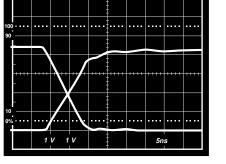
Figure 22. Unloaded Driver Differential Outputs
