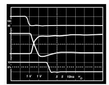
*Figure 25. Driver/Receiver Propagation Delays High to Low*
