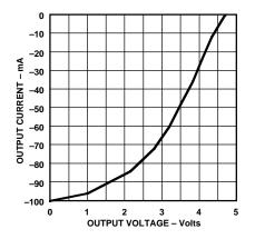
Figure 18. Driver Output High Voltage vs. Output Current
