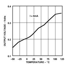
*Figure 14. Receiver Output Low Voltage vs. Temperature*
