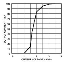
Figure 17. Driver Output Low Voltage vs. Output Current
