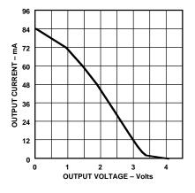
*Figure 15. Driver Differential Output Voltage vs. Output Current*
