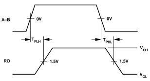
Figure 9. Receiver Propagation Delay
