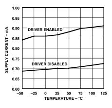
*Figure 19. Supply Current vs. Temperature*
