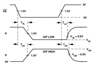
Figure 10. Receiver Enable/Disable Timing
