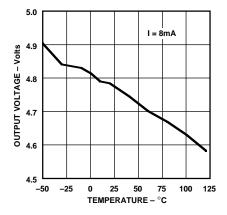
*Figure 13. Receiver Output High Voltage vs. Temperature*
