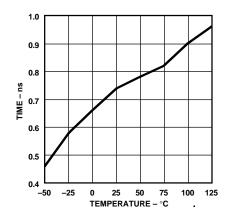
Figure 21. Driver Skew vs. Temperature
