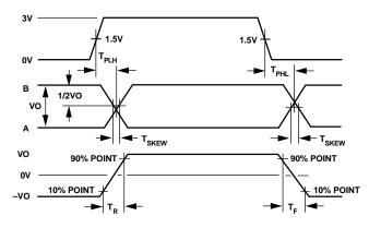
Figure 7. Driver Propagation Delay, Rise/Fall Timing
