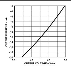
Figure 12. Receiver Output High Voltage vs. Output Current
