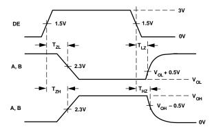
Figure 8. Driver Enable/Disable Timing
