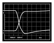
Figure 23. Loaded Driver Differential Outputs
