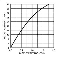
*Figure 11. Receiver Output Low Voltage vs. Output Current*
