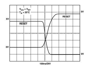
Figure 12. RESET, RESET Assertion
