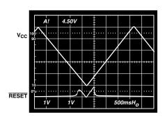
Figure 8. RESET Output Voltage vs. Supply Voltage
