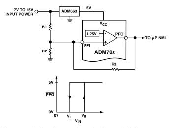
Figure 6. Adding Hysteresis to the Power-Fail Comparator
