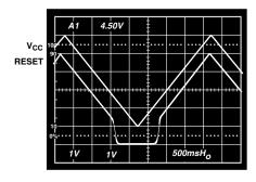
Figure 9. ADM707/ADM708 RESET Output Voltage vs. Supply Voltage
