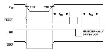
Figure 3. RESET, MR, and WDO Timing
