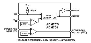
Figure 2. ADM707/ADM708 Functional Block Diagram
