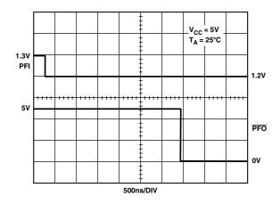
Figure 10. PFI Comparator Assertion Response Time
