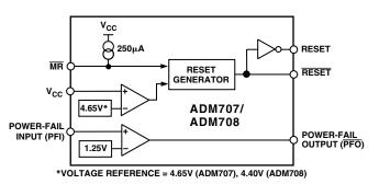
Two supply-voltage monitor levels are available. The ADM705/ADM707 generate a reset when the supply voltage falls below 4.65 V, while the ADM706/ADM708 require that the supply fall below 4.40 V before a reset is issued.
