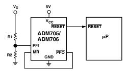
Figure 17. Monitoring 5 V and an Additional Supply,  $V_X$
