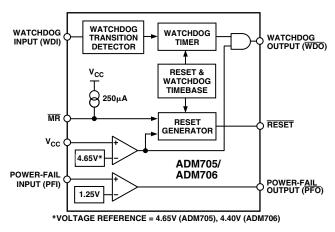
Figure 1. ADM705/ADM706 Functional Block Diagram
