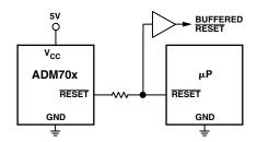
Figure 18. Bidirectional I-O RESET
