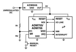
Figure 15. Typical Application Circuit
