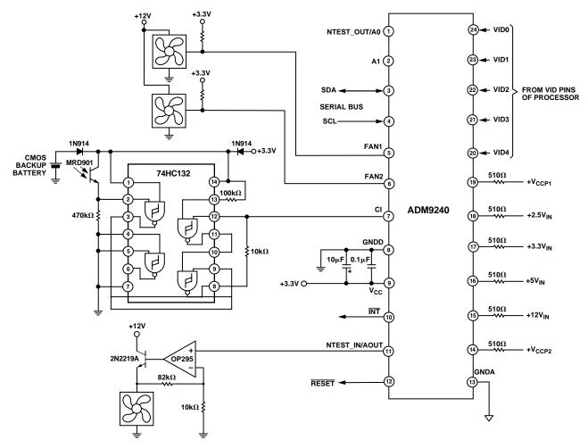
Figure 14. Application Circuit
