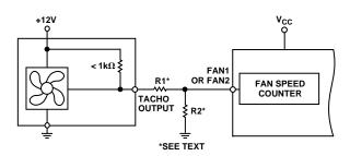
Figure 6d. Fan with Strong Tachometer Pull-Up to  $>V_{CC}$  or Totem-Pole Output, Attenuated with R1/R2
