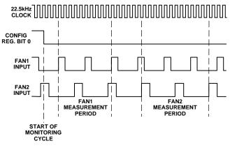
Figure 7. Fan Speed Measurement
