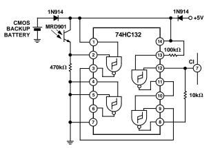
Figure 8a. Chassis Intrusion Detector and Latch
