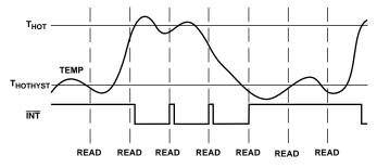
Figure 10. Temperature INT Output in Default Interrupt Mode
