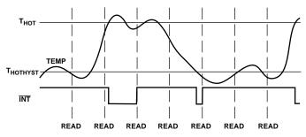
Figure 11. INT Output in One-Time Interrupt Mode
