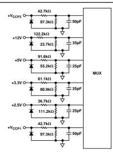
Figure 3. Internal Structure of Analog Inputs
