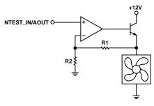
Figure 5. Analog Output Driving Fan
