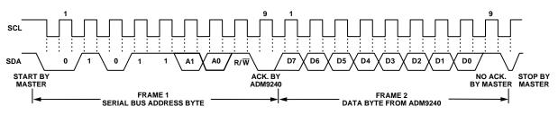
Figure 2c. Reading Data from a Previously Selected Register
