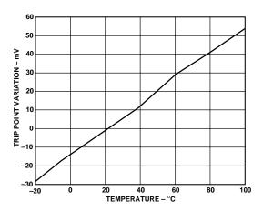
Figure 9. Variation of SU1 High Trip Point With Temperature
