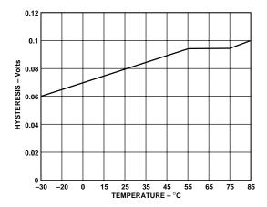
Figure 7. Hysteresis vs. Temperature for SU4—Low to High
