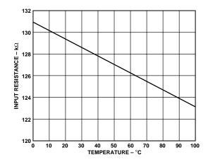
Figure 18. SU2 Input Resistance vs. Temperature
