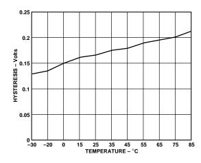
Figure 4. Hysteresis vs. Temperature for SU2—High to Low
