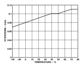
Figure 5. Hysteresis vs. Temperature for SU3—Low to High
