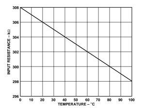
Figure 17. SU1 Input Resistance vs. Temperature
