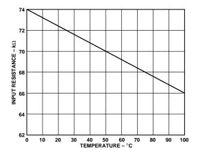
Figure 20. SU4 Input Resistance vs. Temperature
