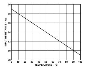
Figure 19. SU3 Input Resistance vs. Temperature
