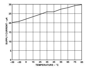
Figure 21. Supply Current vs. Temperature
