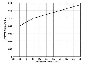
Figure 6. Hysteresis vs. Temperature for SU3—High to Low
