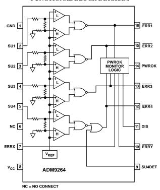
Analog Devices' experience in the design of power supply supervisory circuits is used to provide an optimum solution for the overall circuit in terms of cost, performance and power consumption. Key features of the design include the incorporation of hysteresis and glitch immunity into the comparators, which minimizes the possibility of spurious triggering by noise spikes on the supplies being monitored.
