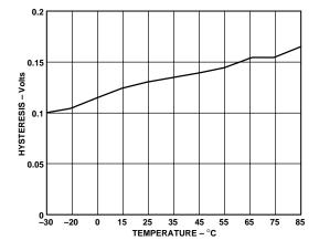
Figure 3. Hysteresis vs. Temperature for SU2—Low to High
