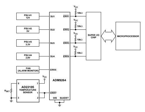
Figure 23. Typical Application of ADM9264
