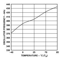
*Figure 9. Oscillator Frequency vs. Temperature*
