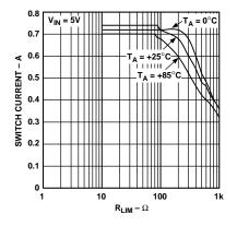
Figure 8a. Maximum Switch Current vs. R<sub>LIM</sub> in Step-Down Mode (5 V)
