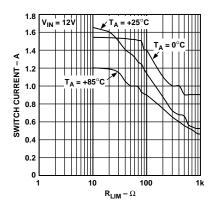
Figure 8b. Maximum Switch Current vs. R<sub>LIM</sub> in Step-Down Mode (12 V)
