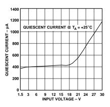
Figure 6. Quiescent Current vs. Input Voltage
