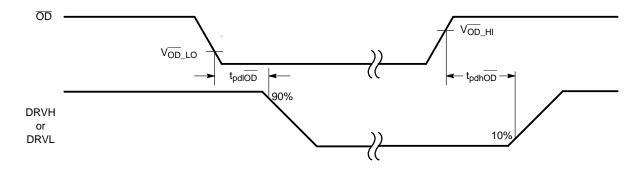
Figure 2. Output Disable Timing Diagram
