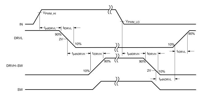
Figure 3. Nonoverlap Timing Diagram
