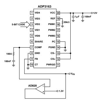
Figure 1. Closed-Loop Output Voltage Accuracy Test Circuit
