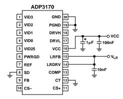
Figure 2. Linear Regulator Output Voltage Accuracy Test Circuit
