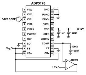
Figure 1. Closed-Loop Output Voltage Accuracy Test Circuit
