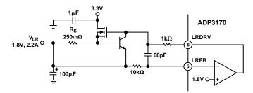
Figure 4. Adding Overcurrent Protection to the Linear Regulator
