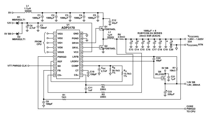
Figure 3. 24 A VRM 8.5-Compliant CPU Supply
