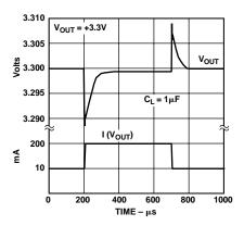
Figure 13. Load Transient for 10 mA to 200 mA Pulse
