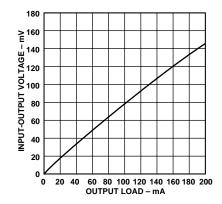
Figure 8. Dropout Voltage vs. Output Current
