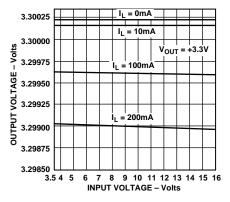
Figure 2. Line Regulation: Output Voltage vs. Supply Voltage
