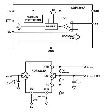
Figure 1. Typical Application Circuit
