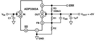
Figure 21. Noise Reduction Circuit
