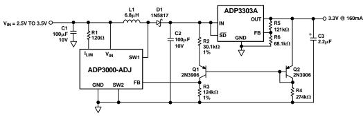
Figure 25. Constant Dropout Post Regulator
