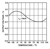
Figure 6. Output Voltage Variation % vs. Temperature
