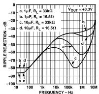
Figure 18. Power Supply Ripple Rejection
