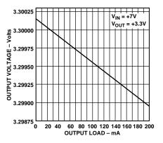
Figure 3. Output Voltage vs. Load Current
