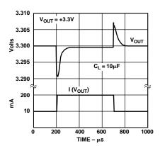
Figure 14. Load Transient for 10 mA to 200 mA Pulse
