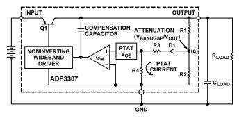
Figure 20. Functional Block Diagram
