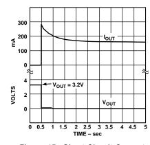
Figure 15. Short Circuit Current
