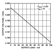
Figure 3. Output Voltage vs. Load Current Up to 100 mA
