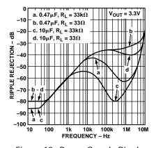
Figure 18. Power Supply Ripple Rejection
