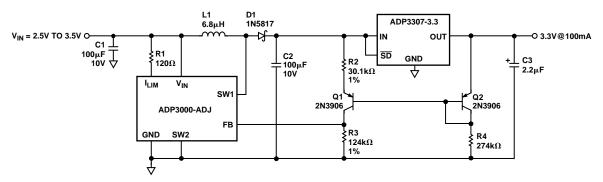
Figure 24. Constant Dropout Post Regulator
