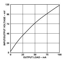
Figure 8. Dropout Voltage vs. Output Current
