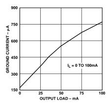
Figure 5. Ground Current vs. Load Current
