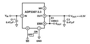
Figure 1. Typical Application Circuit
