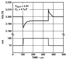
Figure 14. Load Transient
