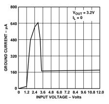
Figure 4. Quiescent Current vs. Supply Voltage—3.2 V (Both Outputs)
