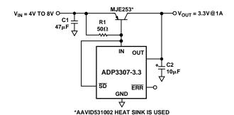
Figure 23. High Output Current Linear Regulator
