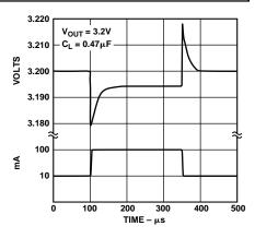
Figure 13. Load Transient
