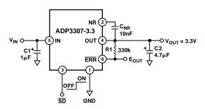
Figure 21. Noise Reduction Circuit
