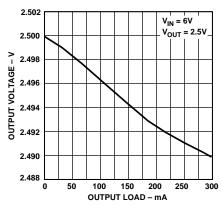
TPC 2. Output Voltage vs. Load Current
