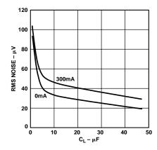
TPC 17. RMS Noise vs.  $C_L$  (10 Hz–100 kHz)
