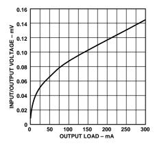
TPC 7. Dropout Voltage vs. Output Current
