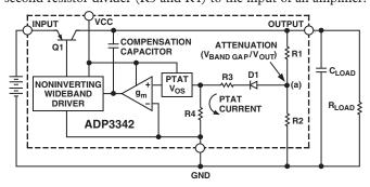
Figure 2. Control Loop Functional Block Diagram
