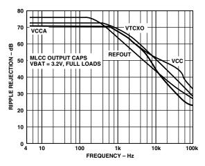
TPC 11. Ripple Rejection vs. Frequency
