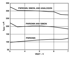
TPC 1. Ground Current vs. Battery Voltage
