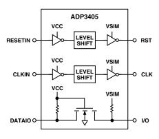
Figure 6. Schematic for Level Translators
