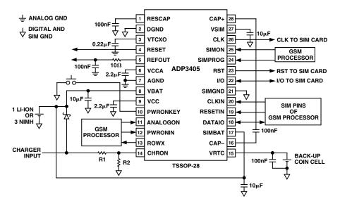
Figure 2. Typical Application Circuit
