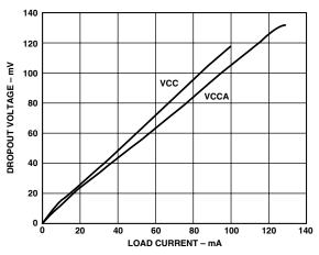
TPC 2. VCC, VCCA Dropout Voltage vs. Load Current
