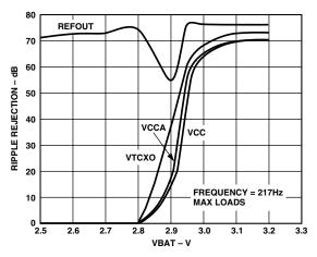
TPC 12. Ripple Rejection vs. Battery Voltage
