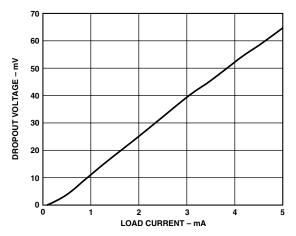
TPC 3. VTCXO Dropout Voltage vs. Load Current
