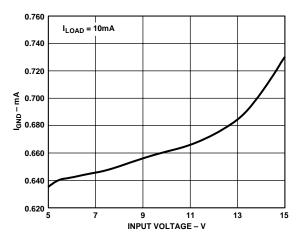
Figure 5.  $I_{GND}$  vs.  $V_{IN}$  ( $I_{LOAD} = 10 \text{ mA}$ )\*
