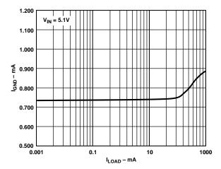
Figure 7.  $I_{GND}$  vs.  $I_{LOAD}$  ( $V_{IN} = 5.1 \text{ V}$ )\*
