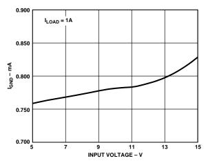
Figure 6.  $I_{GND}$  vs.  $V_{IN}$  ( $I_{LOAD} = 1 A$ )\*
