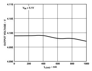
Figure 2.  $V_{OUT}$  vs.  $I_{LOAD}$   $(V_{IN} = 5.1 V)^*$
