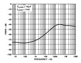
Figure 12. Ripple Rejection\*
