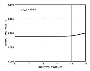
Figure 4.  $V_{OUT}$  vs.  $V_{IN}$   $(I_{LOAD} = 10 \text{ mA})^*$
