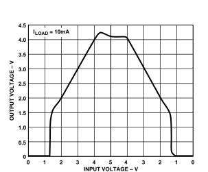
Figure 9. Power-Up/Power-Down\*
