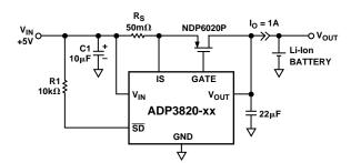
Figure 1. Li-Ion Charger Application Circuit
