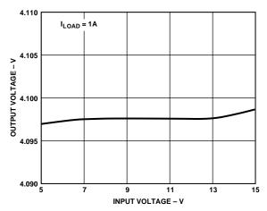
Figure 3.  $V_{OUT}$  vs.  $V_{IN}$  ( $I_{LOAD} = 1 A$ )\*
