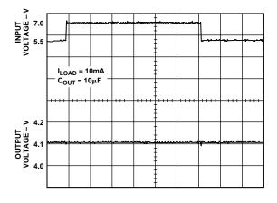
Figure 10. Line Transient Response (10 μF Output Cap)\*
