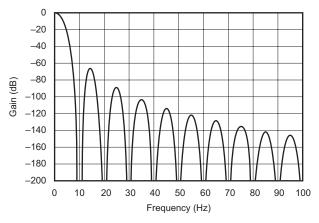
Figure 26. Digital Filter Response (10 Hz)
