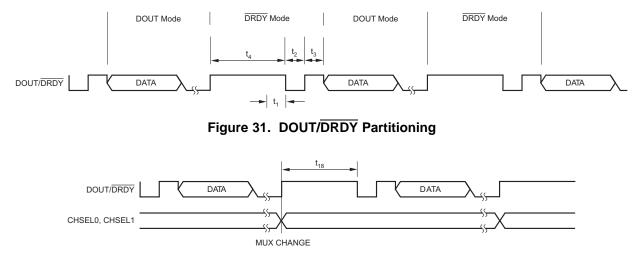
Figure 32. Multiplexer Operation
