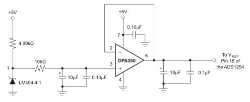
Figure 22. Recommended External Voltage Reference Circuit for Best Low-Noise Operation with the ADS1254
