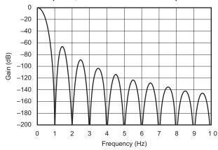
Figure 23. Normalized Digital Filter Response
