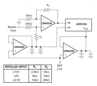
Figure 20. Level Shift Circuit for Bipolar Input Ranges
