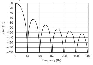
Figure 24. Digital Filter Response (50 Hz)
