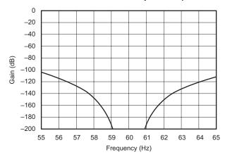
Figure 29. Expanded Digital Filter Response (6 0Hz Figure 30. Expanded Digital Filter Response (60 Hz With a 60-Hz Data Output Rate)
