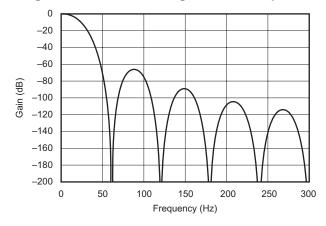
Figure 25. Digital Filter Response (60 Hz)
