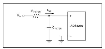
FIGURE 4. RC Input Filtering.
