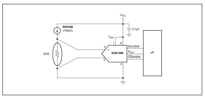
FIGURE 6. ADS1286 with RTD Sensor.
