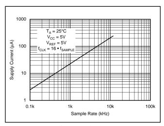
FIGURE 2. Automatic Power Shutdown Between Conversions Allows Power Consumption to Drop with Sample Rate.
