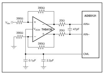
FIGURE 3. DC-Coupled Interface Using Differential I/O Amplifier THS4130.
