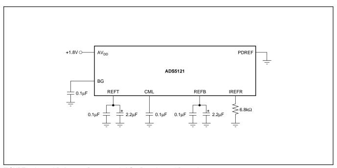
FIGURE 4. Internal Reference; Recommended Configuration and Bypassing.
