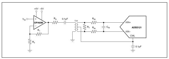
FIGURE 1. Converting a Single-Ended Input Signal into a Differential Signal Using an RF-Transformer.
