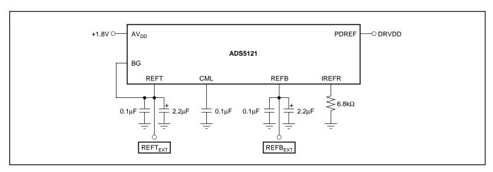
FIGURE 5. External Reference; Recommended Configuration and Bypassing.
