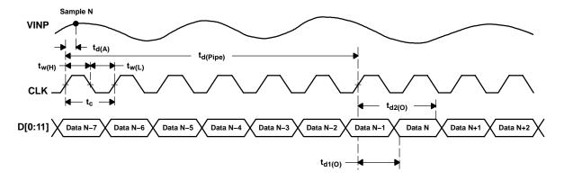
Figure 1. ADS5413 Timing Diagram
