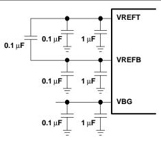
Figure 33. Internal Reference Usage CLOCK INPUTS
