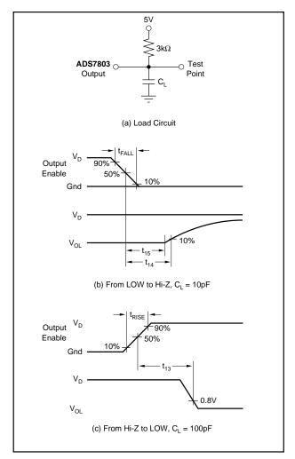
FIGURE 8. Measuring Active LOW to/from Hi-Z State.
