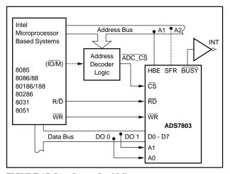
FIGURE 17. Interface to Intel Microprocessors.
