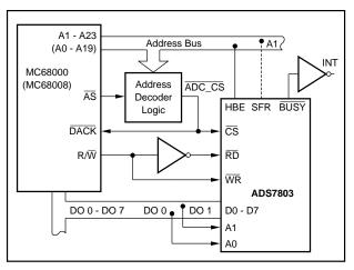
FIGURE 15. Interface to Motorola Microprocessors.
