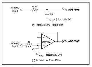
FIGURE 10. Input Signal Conditioning.
