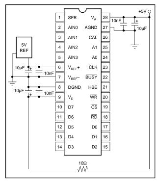
FIGURE 11. Power Supply and Reference Decoupling.
