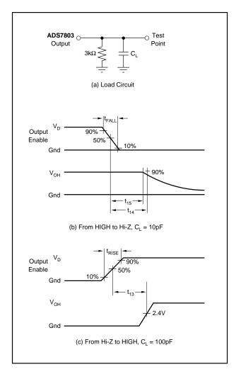
FIGURE 9. Measuring Active HIGH to/from Hi-Z State.
