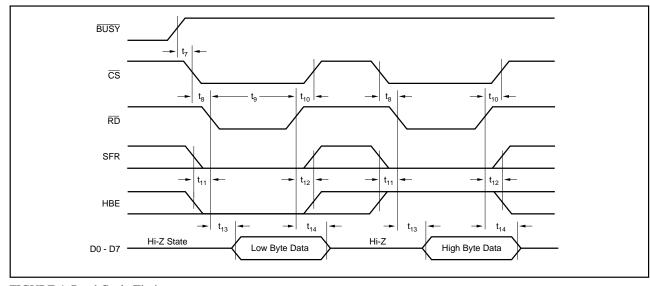
FIGURE 4. Read Cycle Timing.
