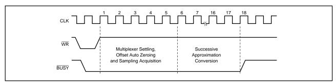
FIGURE 2. Converter Timing.
