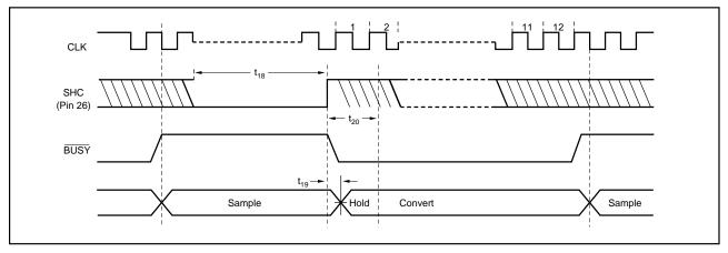
FIGURE 7. Timing for Initiating Conversion in Sample/Hold Control Mode (D2 in SFR HIGH).
