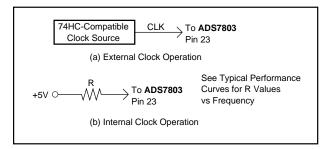
FIGURE 12. Internal Clock Operation.
