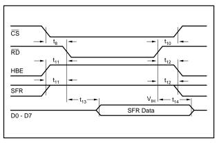
FIGURE 6. Reading the FSR.
