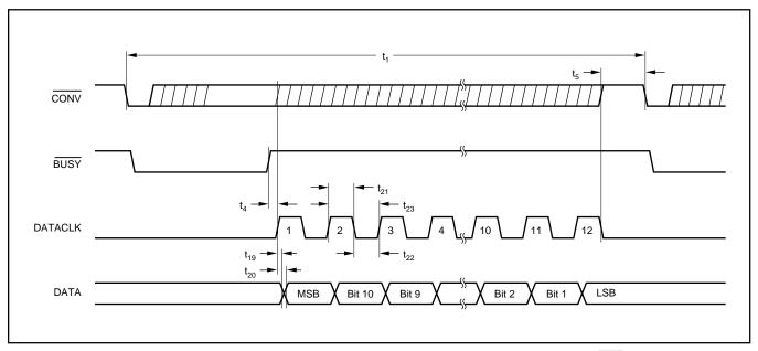
FIGURE 6. Serial Data Timing, External Clock, Clocking After the Conversion Completes (EXT/INT HIGH, CS LOW).
