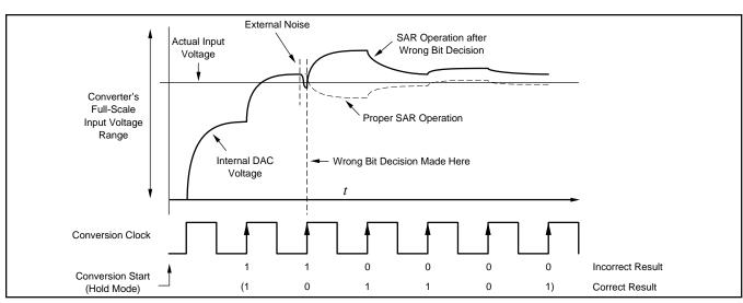
FIGURE 13. SAR Operation When External Noise Affects the Conversion.
