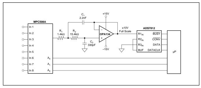
FIGURE 18. Multiplexed Data Acquisition Circuit.
