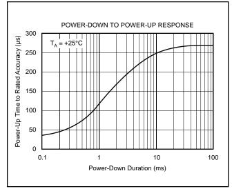
FIGURE 11. Power-Down to Power-Up Response.
