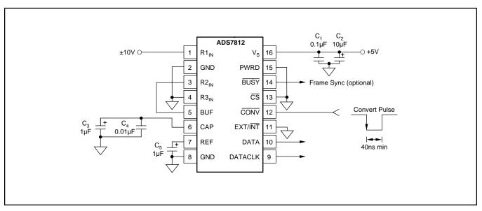
FIGURE 1a. Basic Operation, ±10V Input Range, Internal DATACLK.
