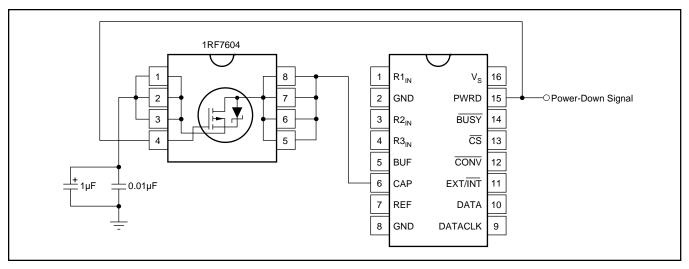
FIGURE 12. Improved Power-Up Response Circuit.
