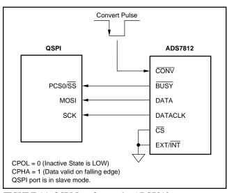
FIGURE 14. QSPI Interface to the ADS7812.
