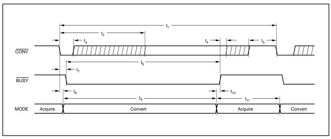
FIGURE 2. Basic Conversion Timing.
