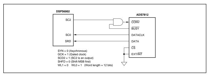
FIGURE 17. DSP56002 Interface to the ADS7812. Processor Initiates Conversions.
