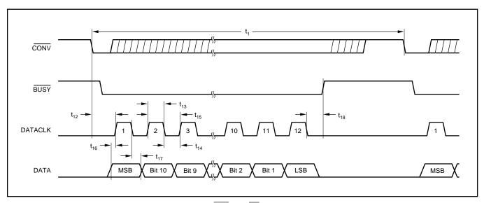
FIGURE 5. Serial Data Timing, Internal Clock (EXT/ $\overline{\text{INT}}$  and  $\overline{\text{CS}}$  LOW).
