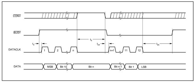
FIGURE 8. Serial Data Timing, External Clock, Clocking After the Conversion Completes and During the Next Conversion (EXT/INT HIGH, CS LOW).
