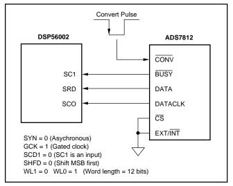
FIGURE 16. DSP56002 Interface to the ADS7812.
