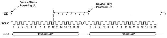
Figure 3. Exiting Power Down Mode
