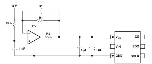
Figure 24. Buffering with the OPA735
