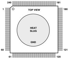
THE 240-LEAD PACKAGE CONTAINS A COPPER HEAT SLUG FLUSH WITH ITS TOP SURFACE. THE SLUG IS EITHER CONNECTED TO GROUND OR FLOATING.
