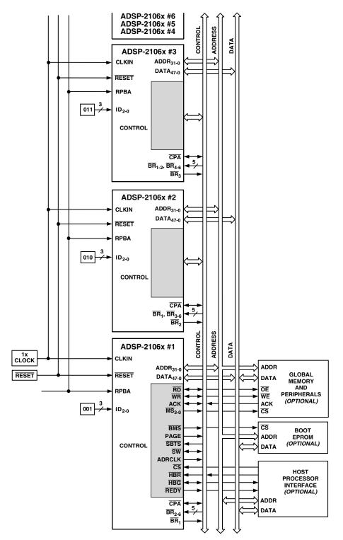
Figure 3. Shared Memory Multiprocessing System
