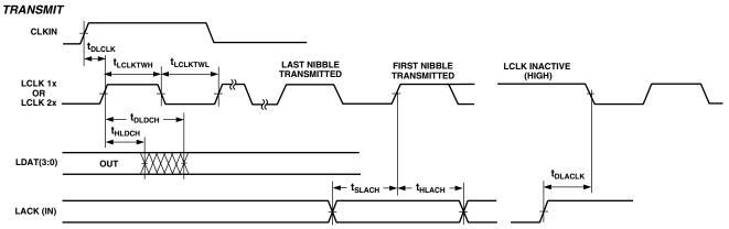
THE **t<sub>slach</sub> requirement applies to the rising edge of LCLK only for the first nibble transmitted.**
