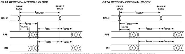
NOTE: EITHER THE RISING EDGE OR FALLING EDGE OF RCLK, TCLK CAN BE USED AS THE ACTIVE SAMPLING EDGE.
