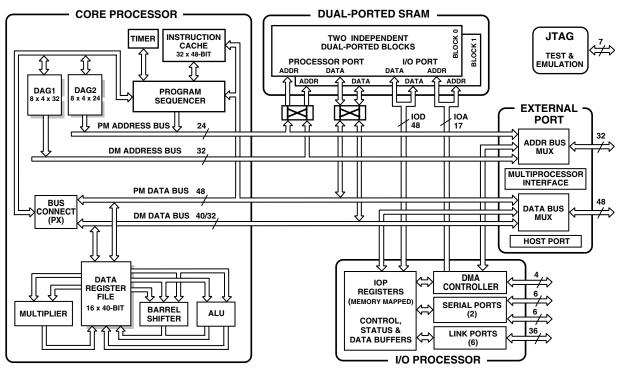
Figure 1. ADSP-21062/ADSP-21062L Block Diagram
