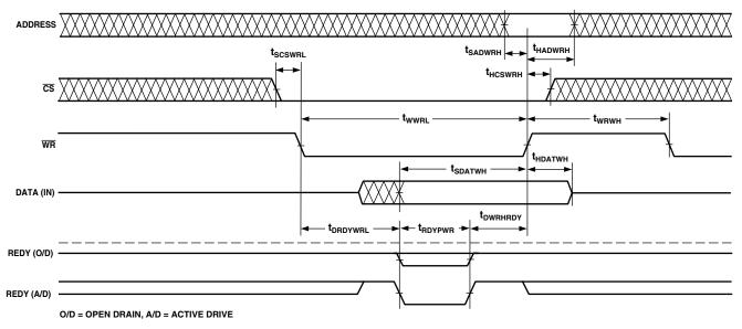
Figure 18b. Asynchronous Read/Write-Host to ADSP-21062
