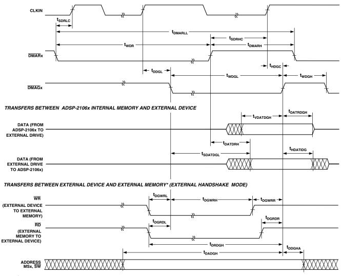
\*MEMORY READ – BUS MASTER, MEMORY WRITE – BUS MASTER, AND SYNCHRONOUS READ/WRITE – BUS MASTER TIMING SPECIFICATIONS FOR ADDR $_{31-0}$ ,  $\overline{RD}$ ,  $\overline{WR}$ ,  $\overline{SW}$ ,  $\overline{MS}_{3-0}$  AND ACK ALSO APPLY HERE.
