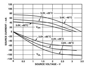
Figure 32. ADSP-21062 Typical Drive Currents (V<sub>DD</sub> = 3.3 V)
