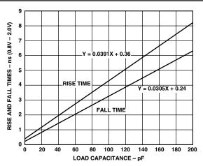
Figure 34. Typical Output Rise Time (0.8 V–2.0 V) vs. Load Capacitance (V<sub>DD</sub> = 3.3 V)
