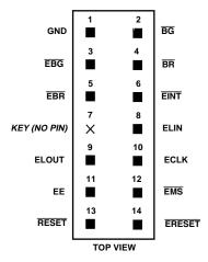
Figure 8. Target Board Connector for EZ-ICE
