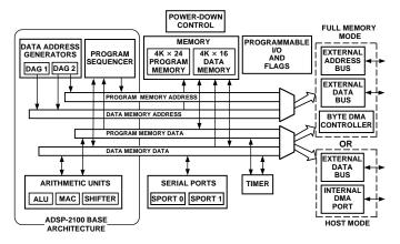
Figure 1. Block Diagram
