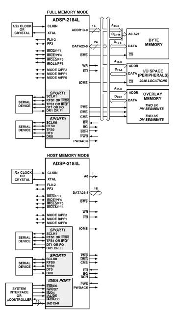
Figure 2. Basic System Configuration
