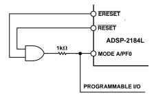
Figure 7. Boot Mode Circuit
