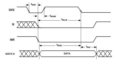
Figure 17. IDMA Write, Long Write Cycle
