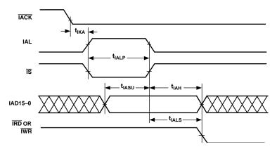
Figure 15. IDMA Address Latch
