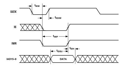
Figure 16. IDMA Write, Short Write Cycle
