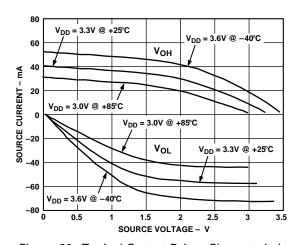
Figure 20. Typical Output Driver Characteristics
