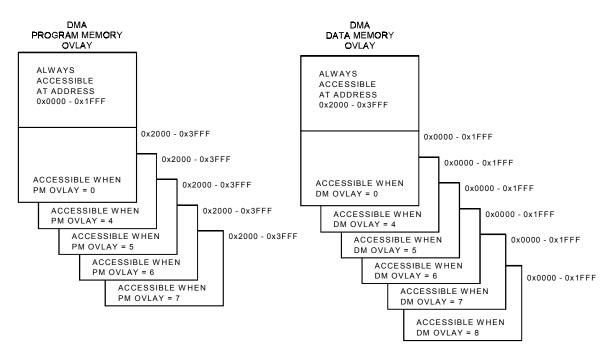
Figure 10. Direct Memory Access - PM and DM Memory Maps
