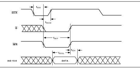
Figure 23. IDMA Write, Short Write Cycle
