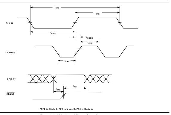
Figure 19. Clock and Reset Signals
