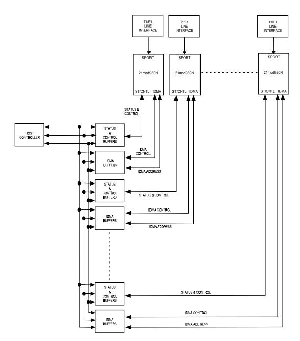
Figure 3. Multichannel Modem Configuration
