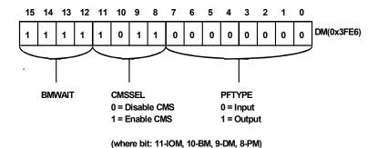
Figure 7. Programmable Flag<sup>1</sup> & Composite Select Control Register
