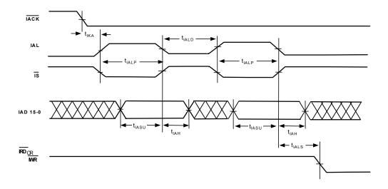
Figure 22. IDMA Address Latch
