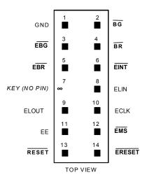
Figure 12. Target Board Connector for EZ-ICE
