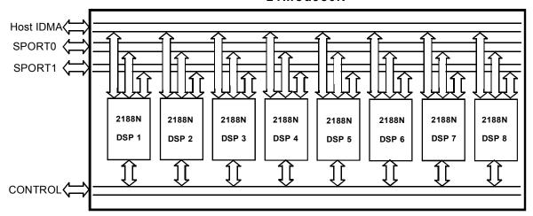
Figure 1. MOD980N MultiPort Internet Gateway Processor Block Diagram
