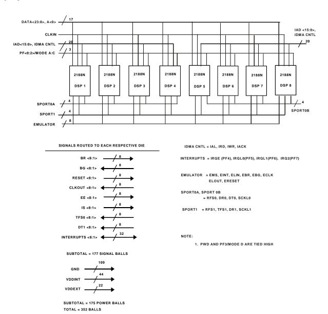
Figure 2. ADSP-21mod980N Functional Block Diagram
