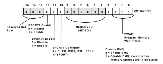
Figure 8. System Control Register
