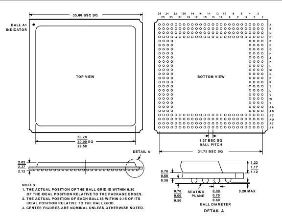
Figure 28. 352-Lead metric Plastic Ball Grid Array (PBGA) (B-352)
