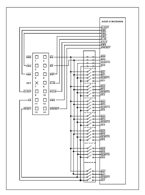
Figure 11. Selecting a Modem Processor in the ADSP-21mod980N
