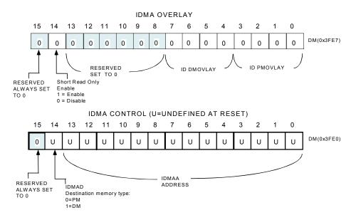
Figure 9. IDMA Control/OVLAY Registers
