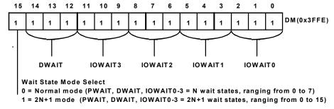
Figure 6. Waitstate Control Register
