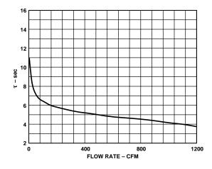
Figure 10. Thermal Response vs. Flow Rate
