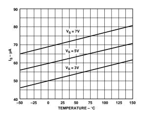
Figure 5. Supply Current vs. Temperature (V<sub>OUT</sub> = HIGH)
