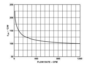
Figure 11. Thermal Resistance vs. Flow Rate
