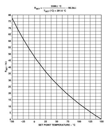
Figure 2. Setpoint Resistor Values
