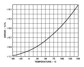
Figure 4. Setpoint Error Due to R<sub>SET</sub> Tolerance
