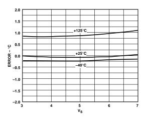
Figure 7. Setpoint Error vs. Supply Voltage
