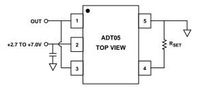
Figure 1. Typical Application Circuit
