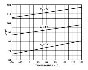
Figure 8. Supply Current vs. Temperature (V<sub>OUT</sub> = LOW)
