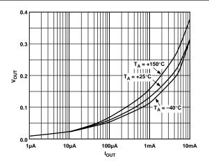
Figure 9.  $V_{OUT}$  vs.  $I_{OUT}$  ( $V_{OUT}$  = LOW)
