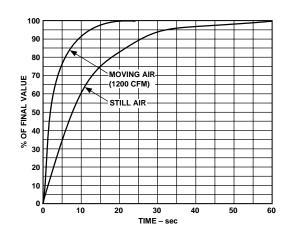
Figure 12. Thermal Response Time
