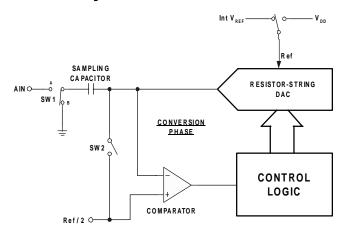
Figure 15. ADC Conversion Phase
