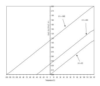
Figure 12. DAC Output vs Temperature, V<sub>REF</sub> = 2.25 V
