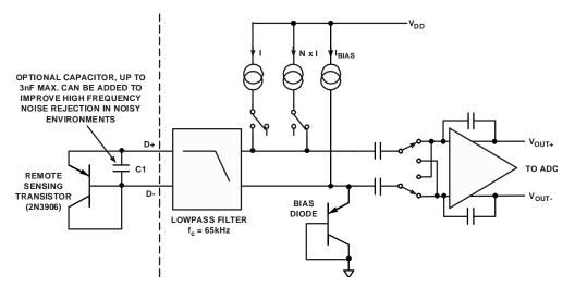
Figure 10. Signal Conditioning for External Diode Temperature Sensor
