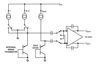
Figure 11. Top Level Structure of Internal Temperature Sensor
