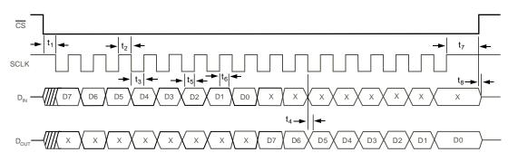
Figure 2. Diagram for SPI Bus Timing
