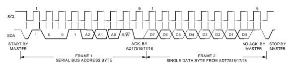
Figure 26. I<sup>2</sup>C - Reading a single byte of data from a selected register
