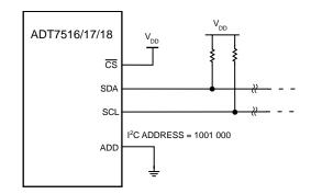
Figure 23(a). Typical I<sup>2</sup>C Interface Connection
