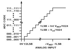
Figure 16. Single-Ended Transfer Function
