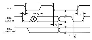
Figure 1. Diagram for I<sup>2</sup>C Bus Timing
