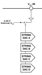
Figure 9. DAC Reference Buffer Circuit
