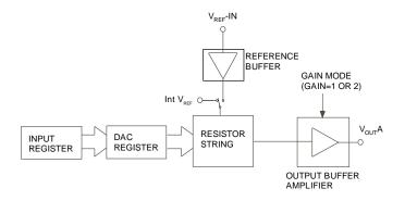
Figure 7. Single DAC channel architecture
