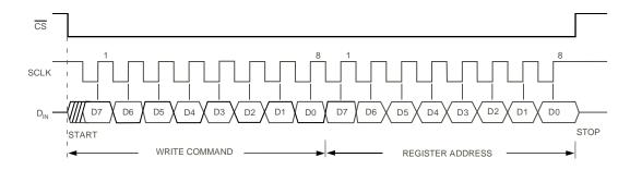
Figure 28. SPI - Writing to the Address Pointer Register to select a register for a subsequent read operation
