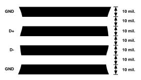
Figure 19. Arrangement of Signal Tracks
