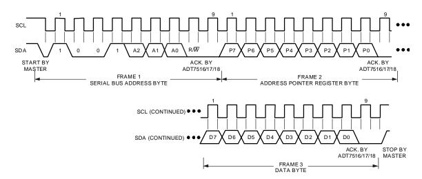
Figure 25. PC - Writing to the Address Pointer Register followed by a single byte of data to the selected register
