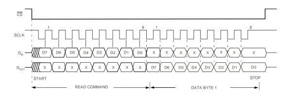
Figure 29. SPI - Reading a single byte of data from a selected register
