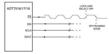
Figure 23(b). Typical SPI Interface Connection
