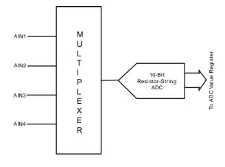
Figure 13. Quad Analog Input Path
