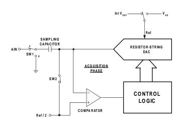
Figure 14. ADC Acquisition Phase
