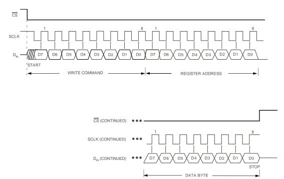
Figure 27. SPI - Writing to the Address Pointer Register followed by a single byte of data to the selected register
