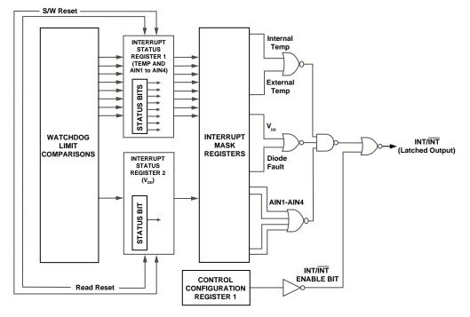
Figure 18. ADT7516/17/18 Interrupt Structure
