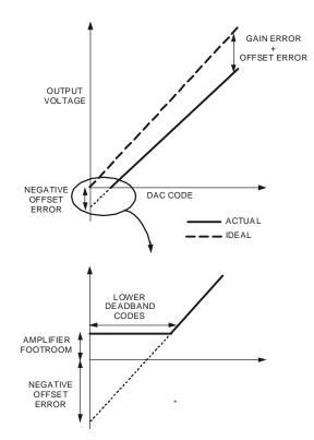
Figure 5. DAC Transfer Function with Negative Offset
