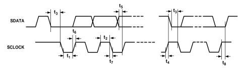
Figure 1. MPU Port Timing Diagram
