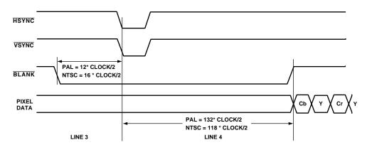
Figure 22. Timing Mode 2 Even-to-Odd Field Transition
