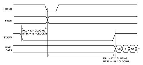
Figure 19. Timing Mode 1 Odd/Even Field Transitions
