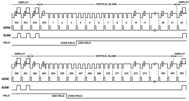
Figure 24. Timing Mode 3 (NTSC)
