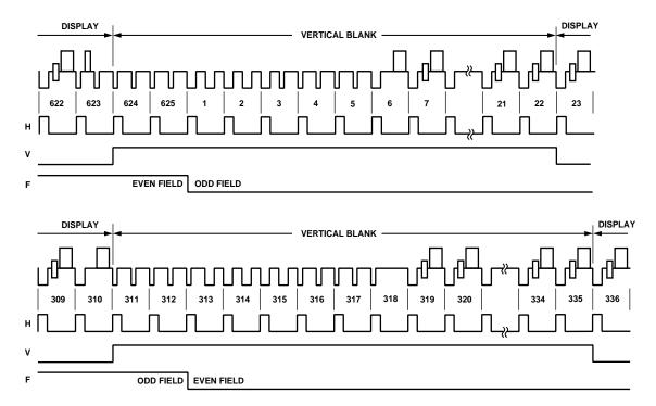
Figure 15. Timing Mode 0 (PAL Master Mode)
