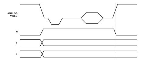
Figure 16. Timing Mode 0 Data Transitions (Master Mode)
