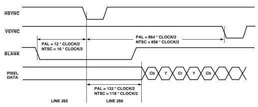
Figure 23. Timing Mode 2 Odd-to-Even Field Transition
