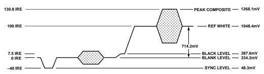
Figure 44. NTSC Composite Video Levels
