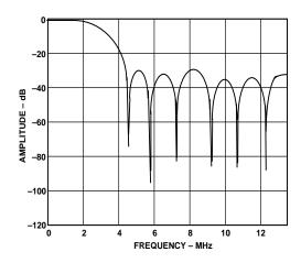
Figure 8. PAL Notch Filter
