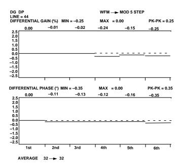
Figure 61. Differential Phase and Gain Measurements (PAL)
