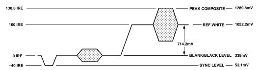
Figure 48. NTSC Composite Video Levels
