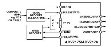
Figure 12. RTC Connections
