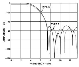
Figure 5. NTSC Low-Pass Filter
