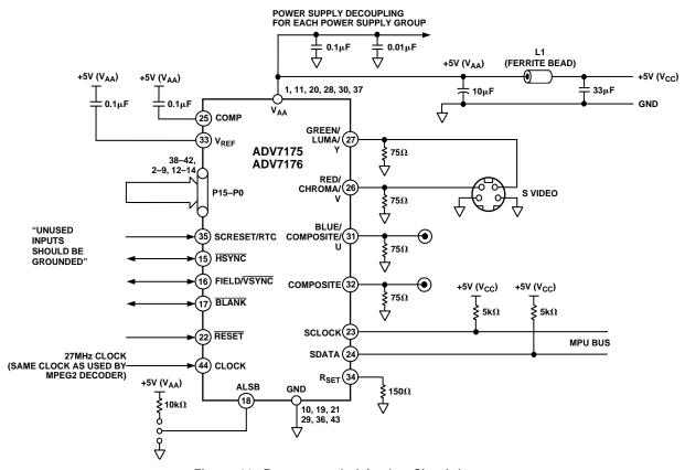
Figure 41. Recommended Analog Circuit Layout
