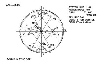
Figure 62. Vectorscope Measurements (PAL)
