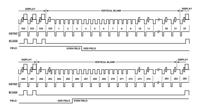
Figure 17. Timing Mode 1 (NTSC)
