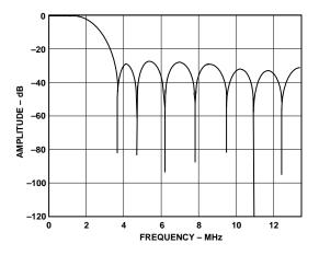
Figure 6. NTSC Notch Filter
