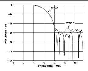
Figure 7. PAL Low-Pass Filter
