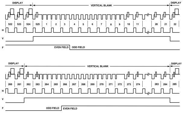
Figure 14. Timing Mode 0 (NTSC Master Mode)
