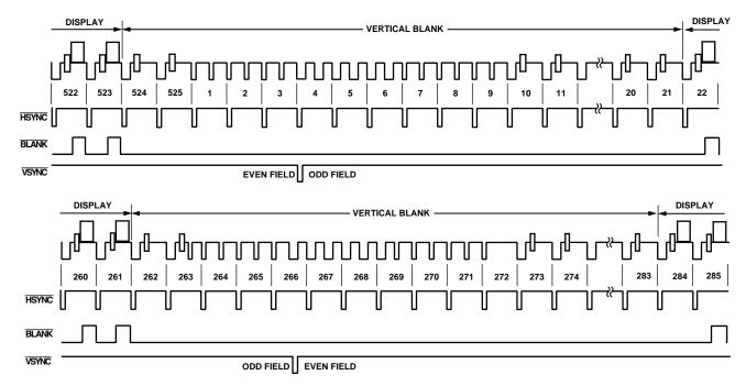
Figure 20. Timing Mode 2 (NTSC)
