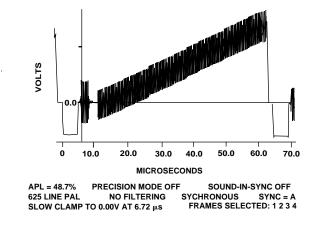
Figure 63. Modulated Ramp Measurements (PAL)
