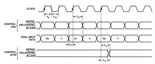
Figure 2. Pixel and Control Data Timing Diagram
