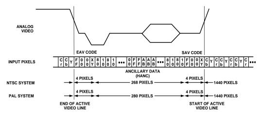
Figure 13. Timing Mode 0 (Slave Mode)
