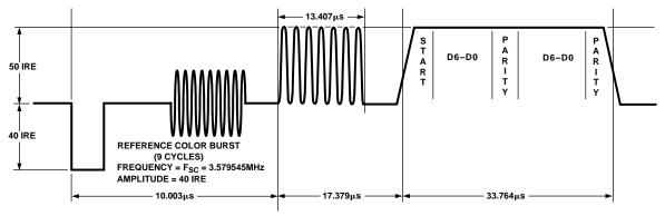
Figure 43. Closed Captioning Waveform (NTSC)
