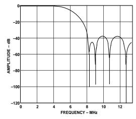
Figure 9. NTSC/PAL Extended Mode Filter
