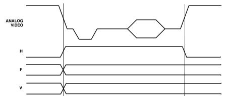
Figure 10. Timing Mode 0 Data Transitions (Master Mode)
