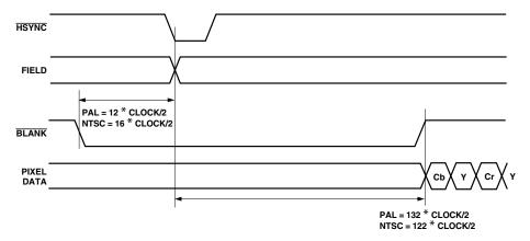
Figure 13. Timing Mode 1 Odd/Even Field Transitions Master/Slave
