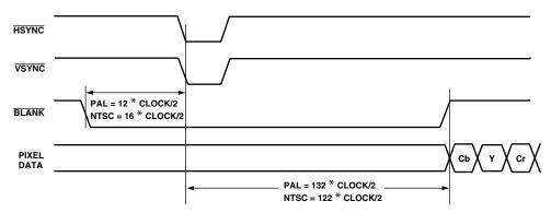
Figure 16. Timing Mode 2 Even-to-Odd Field Transition Master/Slave
