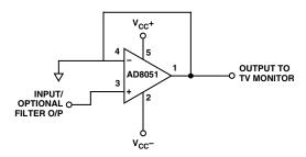
Figure 59. Recommended Output DAC Buffer
