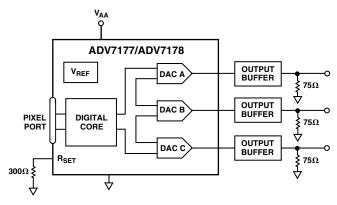
Figure 58. Output DAC Buffering Configuration
