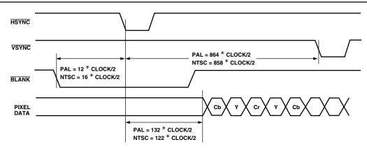
Figure 17. Timing Mode 2 Odd-to-Even Field Transition Master/Slave
