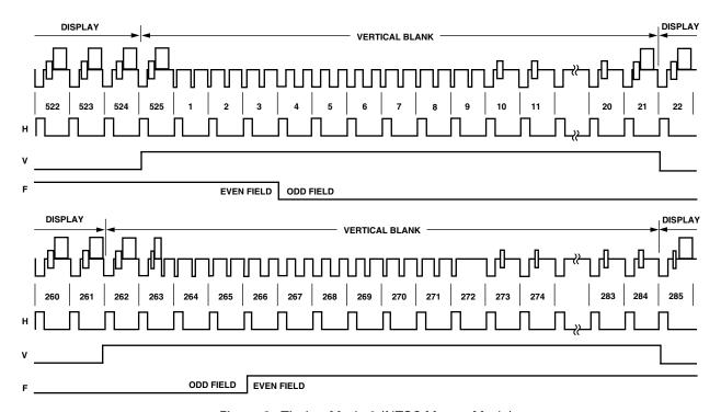
Figure 8. Timing Mode 0 (NTSC Master Mode)
