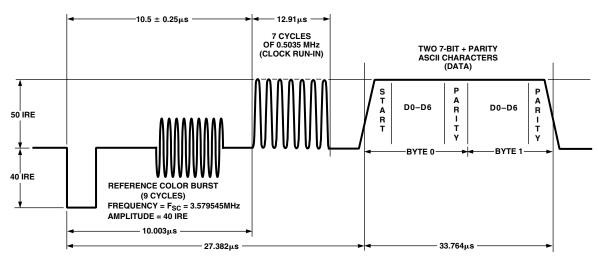
Figure 37. Closed Captioning Waveform (NTSC)
