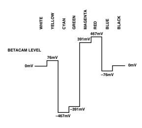
Figure 54. NTSC 100% Color Bars with Pedestal V Levels
