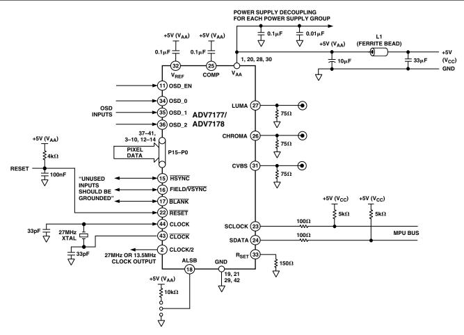
Figure 36. Recommended Analog Circuit Layout
