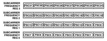
Figure 27. Subcarrier Frequency Register
