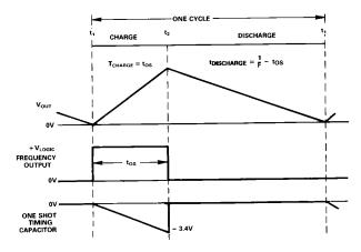
Figure 2. Voltage-to-Frequency Conversion Waveforms
