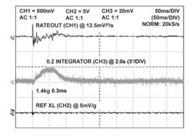
Figure 17. Hi-g Shock in Rate Axis (40 Hz)
