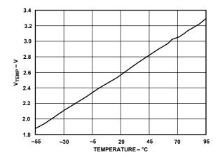
Figure 5. Temperature Sensor Output
