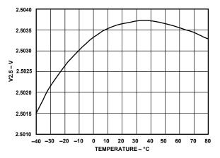
Figure 8. 2.5 V Voltage Reference vs. Temperature
