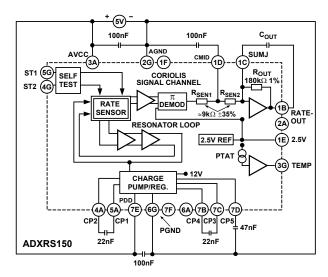
Figure 22. Block Diagram with External Components
