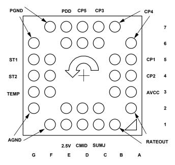
Figure 27. BGA-32 (Bottom View)
