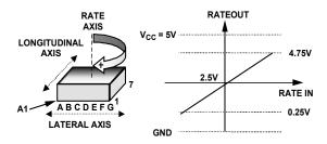
Figure 2. RATEOUT Signal Increases with Clockwise Rotation
