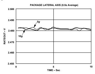
Figure 12. 10 g Random Vibration in Package-Lateral Axis Orientation
