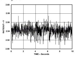
Figure 23. Random Vibration (Lateral) 10 kHz to 20 kHz at 0.01 g/ $^{\parallel}$ Hz with 60 Hz Sampling and 0.5 Sec Averaging
