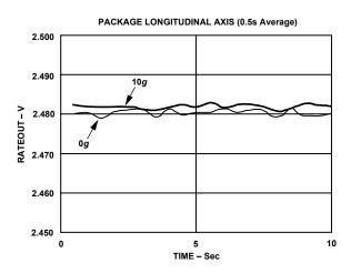
Figure 13. 10 g Random Vibration in Package-Longitudinal Axis Orientation
