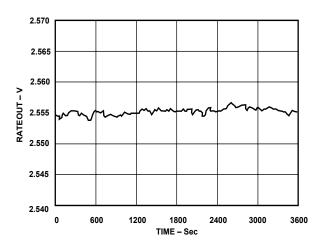
Figure 4. Null Stability for 1 Hour
