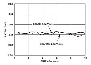
Figure 25. Random Vibration (Lateral) 10 kHz to 20 kHz at 0.01 g/ $\sqrt{\text{Hz}}$  with 60 Hz Sampling and 0.5 Sec Averaging
