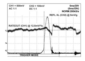
Figure 18. Shock Test 100 g, 5 ms in Longitudinal Axis (40 Hz)
