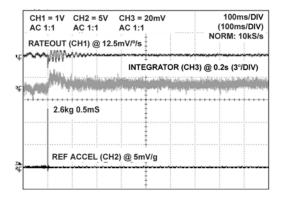
Figure 19. Hi-g Shock Test, Lateral Axis, 10× Time Base (40 Hz)
