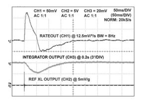
Figure 20. Hi-g Shock, Rate Axis, BW Reduced to 8 Hz
