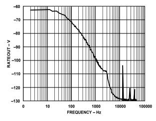
Figure 26. Noise Spectral Density at RATEOUT –BW = 4Hz
