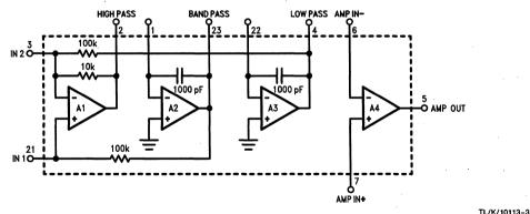
FIGURE 1. AF151 Schematic (Section 1)
