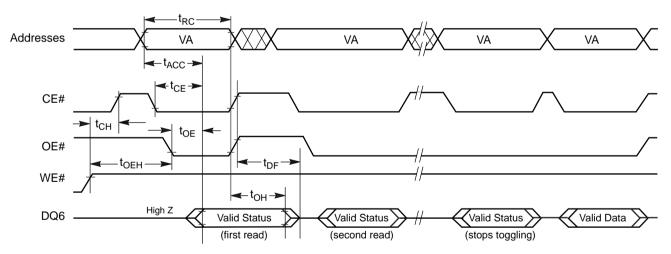
**Note:** VA = Valid address; not required for DQ6. Illustration shows first two status cycle after command sequence, last status read cycle, and array data read cycle.
