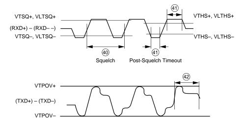
Figure 6. 10BASE-T Interface Timing Diagram
