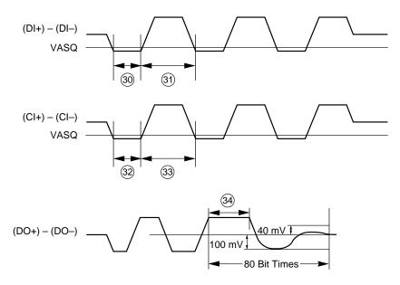
Figure 5. AUI Timing Diagram
