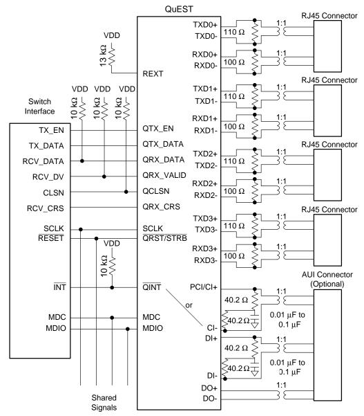
**Note:** If <u>QINT</u> and the AUI port are used, a special circuit (not shown) is needed for PCI. Optional 10K resistors are used to set internal address match for Management Address.
