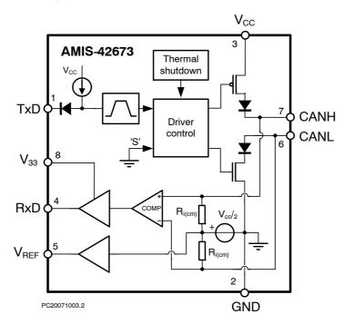
Figure 1. Block Diagram
