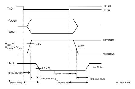
Figure 6. Timing Diagram for AC Characteristics
