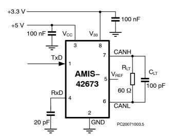
Figure 5. Test Circuit for Timing Characteristics
