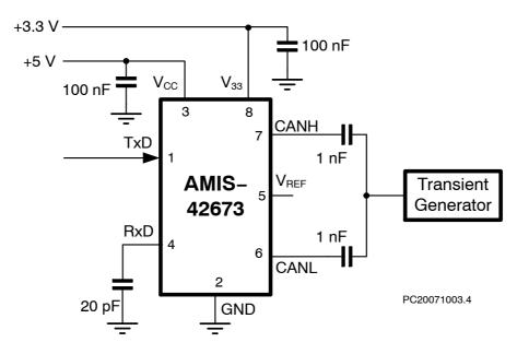
**Figure 3. Test Circuit for Automotive Transients**
