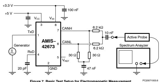
Figure 7. Basic Test Setup for Electromagnetic Measurement
